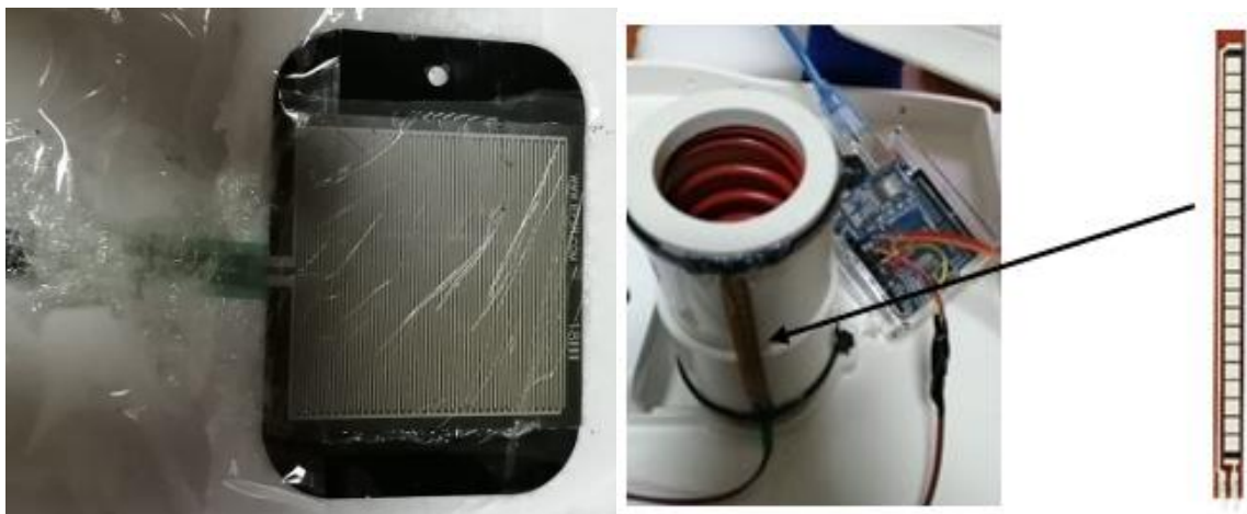
Figure 6. Placing Force And Flex Sensors In The Manikin
