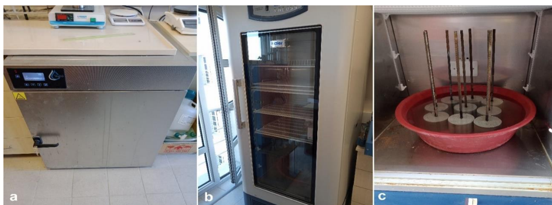
Figure 4. Stove (a) and refrigerator (b and c) used in this study
