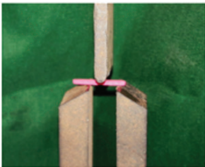
Figure 4. Three-point bend test for flexural strength evaluation.
