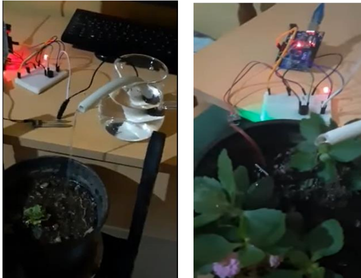
Photo 2. Irrigation system with Arduino
