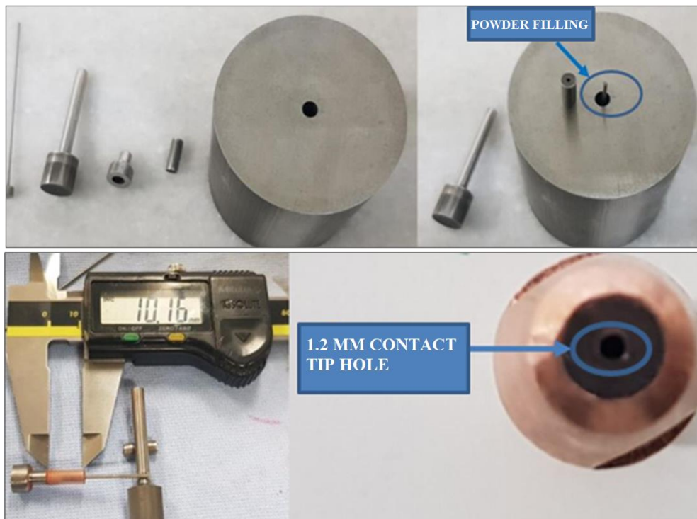
Figure 2. Contact guide pin in compression die (Above); image of compressed pin (Left-Below) in contact guide pin (Right-Below). In terms of the way the die is made, a pin passes through its middle and forms the inner hole of the contact tip.
