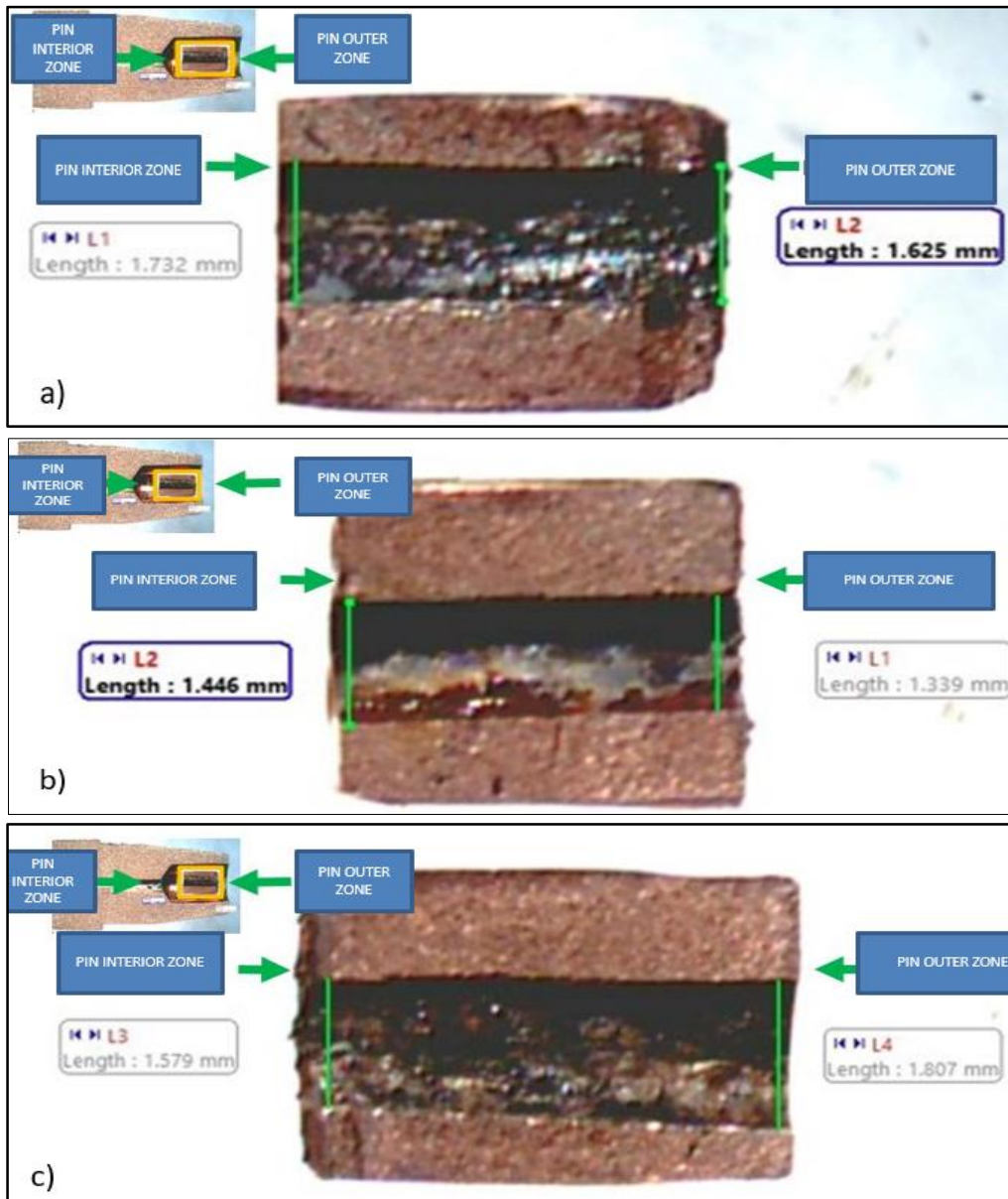
Figure 9. Close-up image of the cross-section of the contact guide (pin) a)CuW15, b)CuW10 and c)CuW5) tested in mass production.
