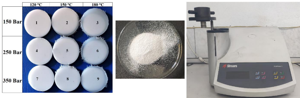
Figure 1. Macrostructure photographs of the produced samples, UHMWPE powder, and hot molding device used in experiments
