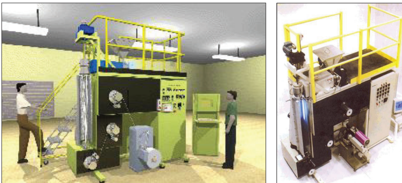
Figure 6. Hills Lab-Type Filament Yarn Machine (Fiber Extrusion Research&Pilot Machines for Homo&Bicomponent Laboratory Applications, 2022)
