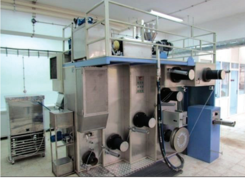
Figure 13. Image of Developed Lab-Type Filament Drawing Machine (LabFil) (Hacıoğulları Özkan and Babaarslan, 2015)
