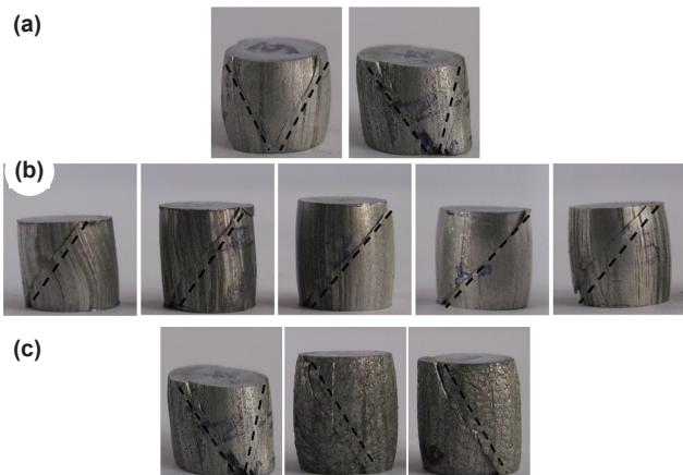
Figure 9. Fracture behavior of materials subjected to compression test, a) Semi-brittle fracture behavior of Al2124 and Al2124-B 4 C (5%), b) Brittle fracture behavior of Al7075, Al7075-Al2124, Al7075-Al2124-B 4 C (5%), Al7075-Al2124-B 4 C (10%) and Al7075-Al2124 (15%), c) Fracture behavior of Al2124-B 4 C (5%), Al2124-B 4 C (10%) and Al2124-B 4 C (15%).
