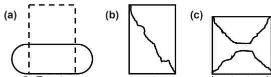
Figure 8. Fracture types seen at compression tests a) Failure by barreling, b) Brittle fracture, c) Semi-brittle fracture.
