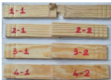
Scotch pine wood- PVA wood glue - no additives
