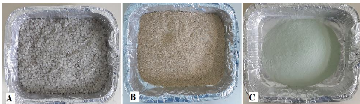
Figure 1. Recycled polyethylene (A), pine wood flour (B), waste glass flour (C)
