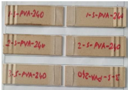
PLA Wood- PVA wood glue - no additives
