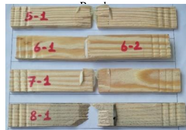
Scotch pine wood- Loctite 9466- no additives
