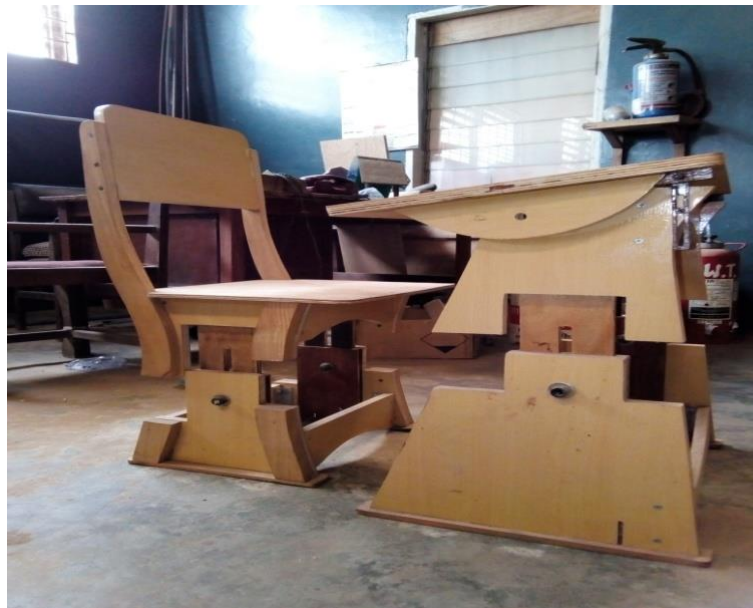
Figure 2. Sitting-posture Measurement Device (Developed by MWP Lab 2015)
