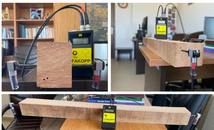
Figure 1. Determination of time of flight on beech timber
