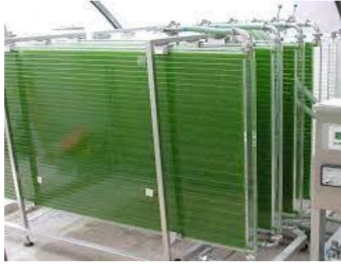
Figure 4. Flat-panel photobioreactor production system (Kükdamar & Tokuç 2015).
