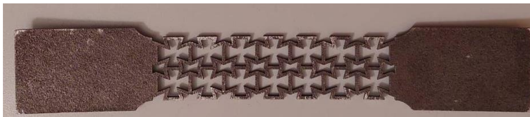
Figure 2. Tensile auxetic sample produced from AlSi10Mg by DMLS method
