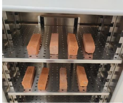
Figure 3. Drying the samples in an furnace
