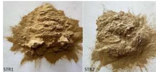
Figure 1. Powdered form of struvites recovered from liquid fermented product
