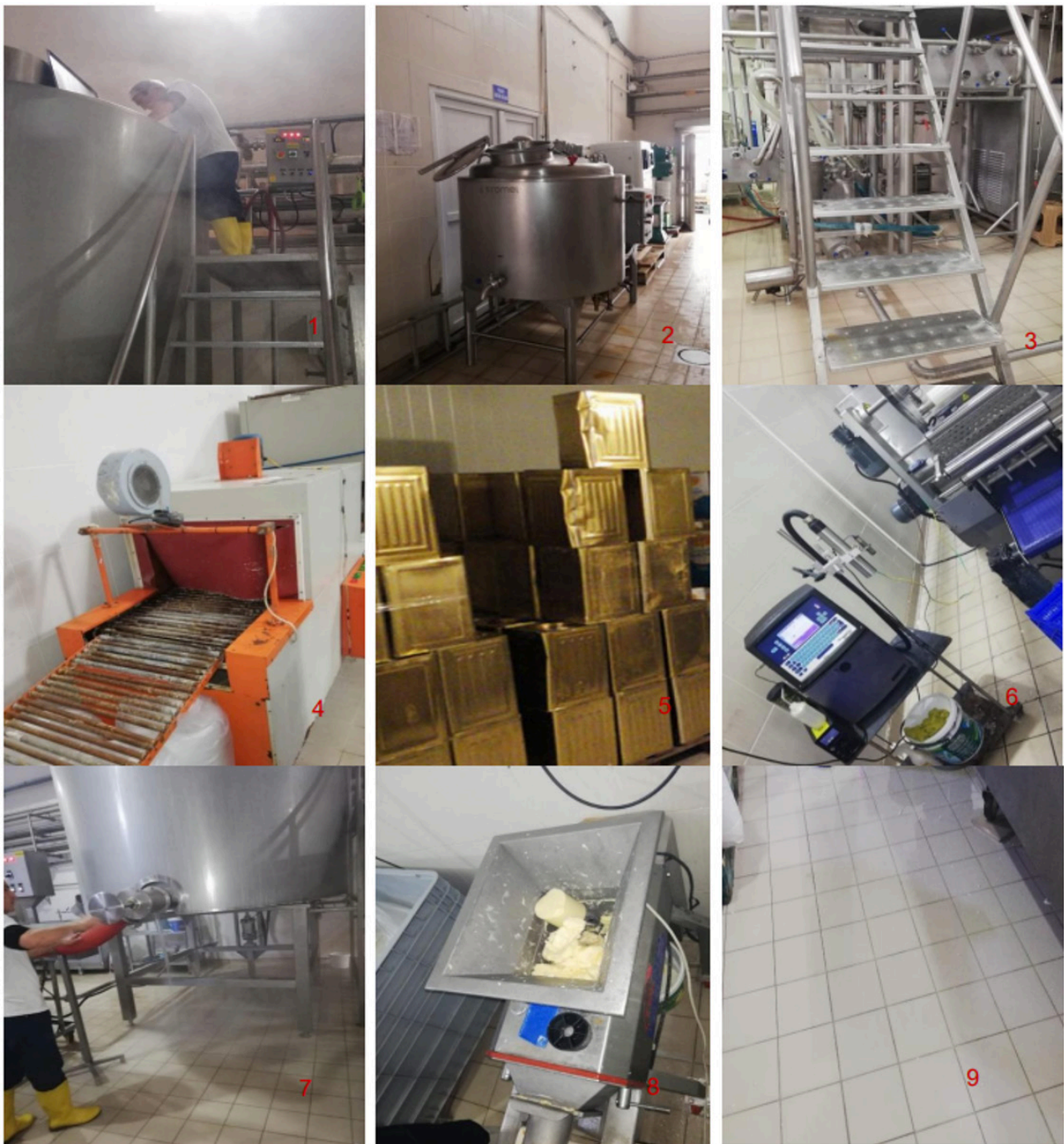
Figure 3. Photographic report on working environment hazards. The different risks identified are illustrated in the photographic report. Physical and ergonomic risk. Physical and ergonomic risk (1,2,3), ergonomic risk (2,4,5), accident risk (1,8,9), physical risk (1,2,5,7) and (9), physical and accident risk (1,2,3,4,6), accident risk (8), hygiene risk (6).
