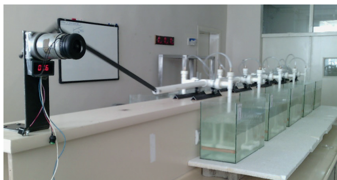
Figure 2. Sediment suspension apparatus used in the experiments: drive mechanism, drive shaft cross coupling, and arm (Original).
