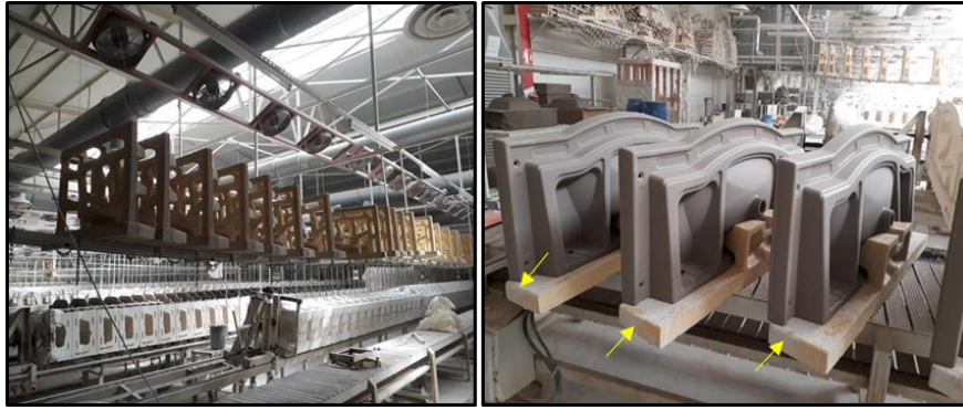
Figure 1. Examples of RPU materials used as a modeling support apparatus in production of ceramic sanitary ware
