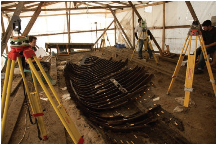
F. 4: Measurements using Total Station® (IU Yenikapı Shipwrecks Project Archive, 2008)
