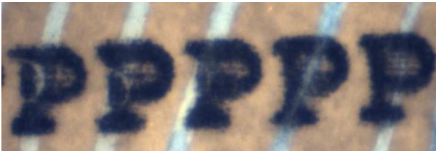
Figure 4. Interruption of luminescence of ballpoint pen ink stroke, when non luminescent typewritten stroke was above luminescent ballpoint pen ink stroke. The typewritten stroke forms thick layer over the ballpoint pen ink stroke which mask the luminescence of ballpoint pen ink stroke.
