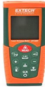
Figure 2. Extech DT300 Laser meter. Şekil 2. Extech DT300 Lazermetre.
