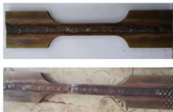
Figure 1 Photograph showing the failure location in AISI 410 stainless steel welded with TIG
