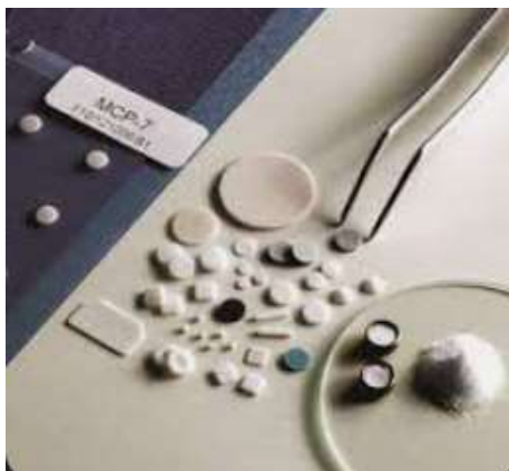
Figure 1. Types of TLD dosimeters
