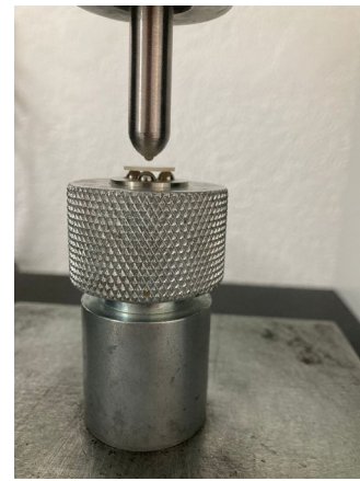
Figure 1. Machine for biaxial flexural testing with a disc-shaped specimen.
