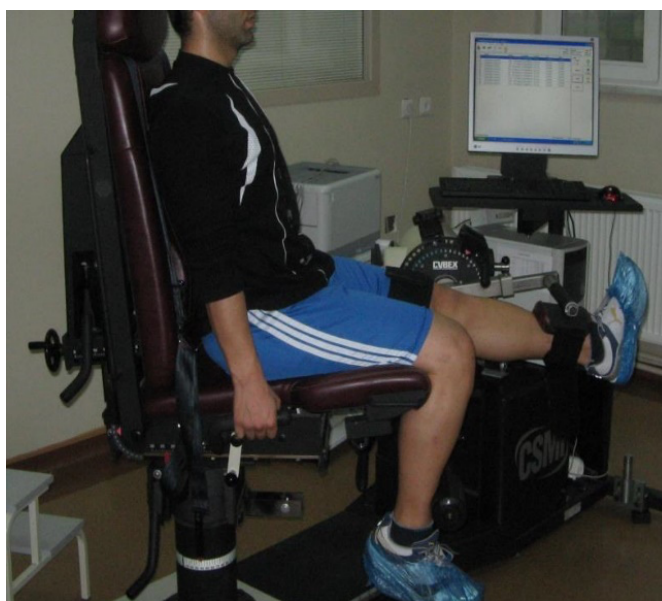
Fig. 2. Measurement of muscle strength and proprioception with the HUMAC NORM II® isokinetic dynamometer.
