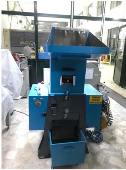
Figure 2. Blade mill shredder.
