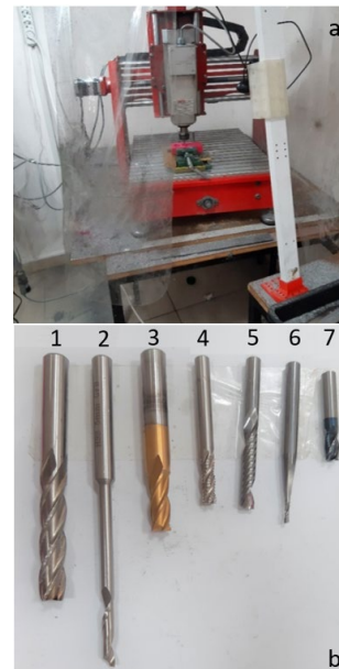
Figure 4. a) Desktop CNC milling machine b) end milling cutters used in processing.
