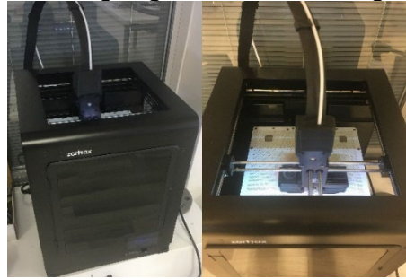
Figure 3. 3D Additive manufacturing equipment.
