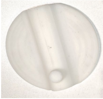
Figure 10. Additive manufacturing mould.
