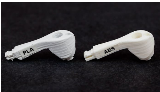
Figure 2. 3D printed samples appearance [26].
