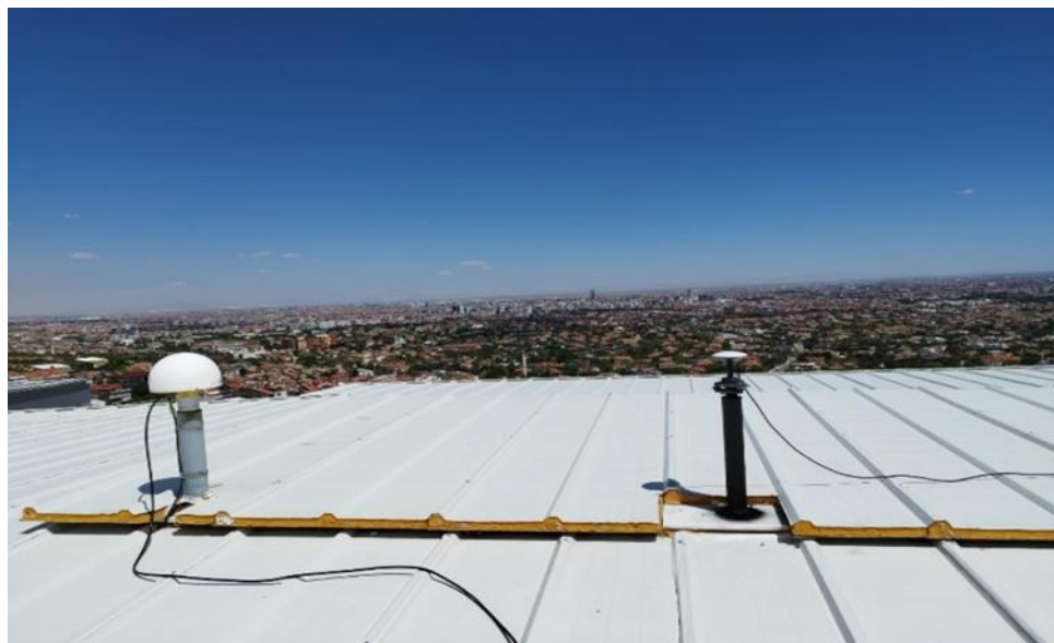
Figure 1. The u-blox and geodetic-grade antennas, which were placed on the Faculty of Engineering, Necmettin Erbakan University
