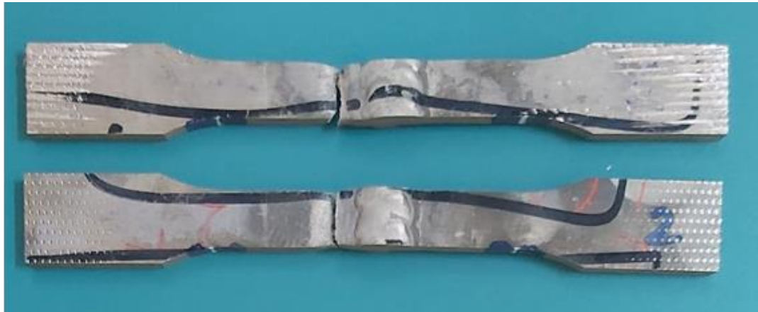
Figure 7. Failure zones of the GTAWed samples after tensile testing
