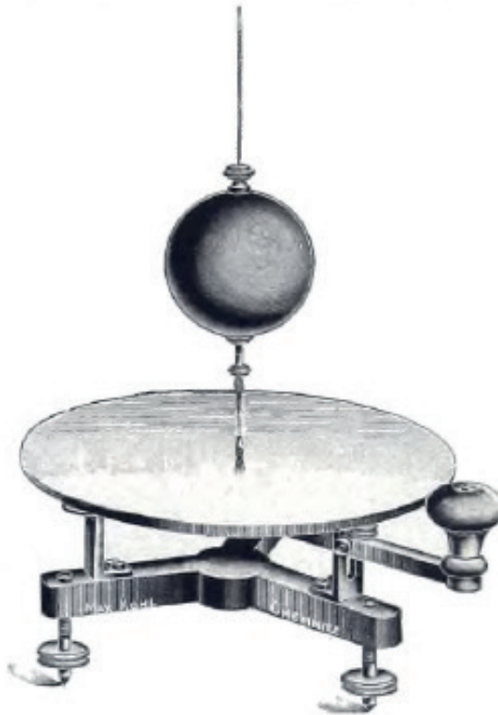
Image 9. Weinhold's apparatus for Foucault's pendulum made by Max Kohl. 27
