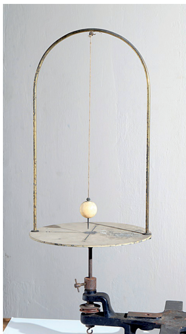
Image 4. Small pendulum for demonstrating the principles of Foucault's experiment from the collection of the College (Photo: P. Lazos).
