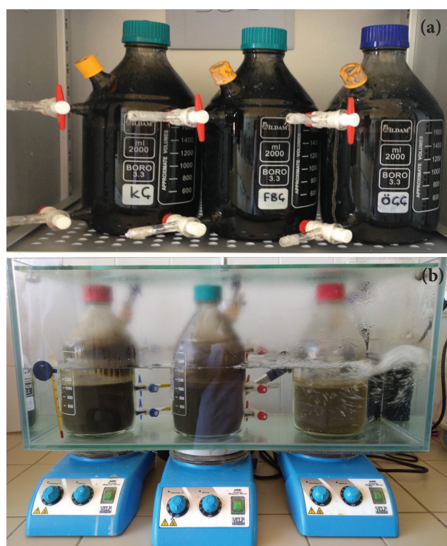
Figure 1. Lab-scale anaerobic digesters (a) IM and (b) CM modes.
