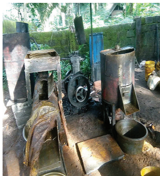
Figure 2. The palm oil mills showing palm nut digester, nut and pulp separator and the diesel-powered engine.
