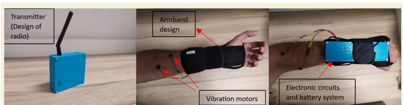
Figure 5. Components of the designed armband
