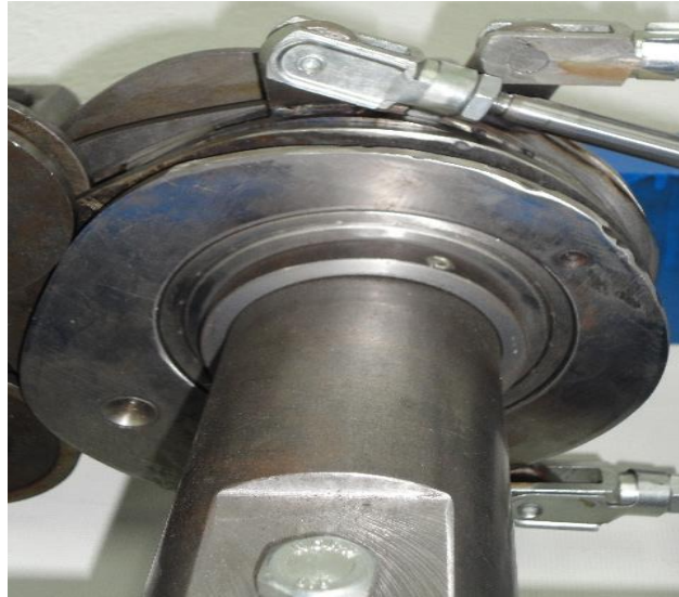
Figure 2. Fixed Shedding Status of Cams
