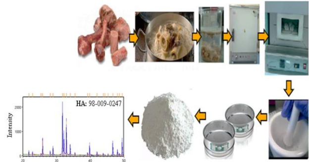
Figure 1. Schematic presentation of the production of SHA powder
