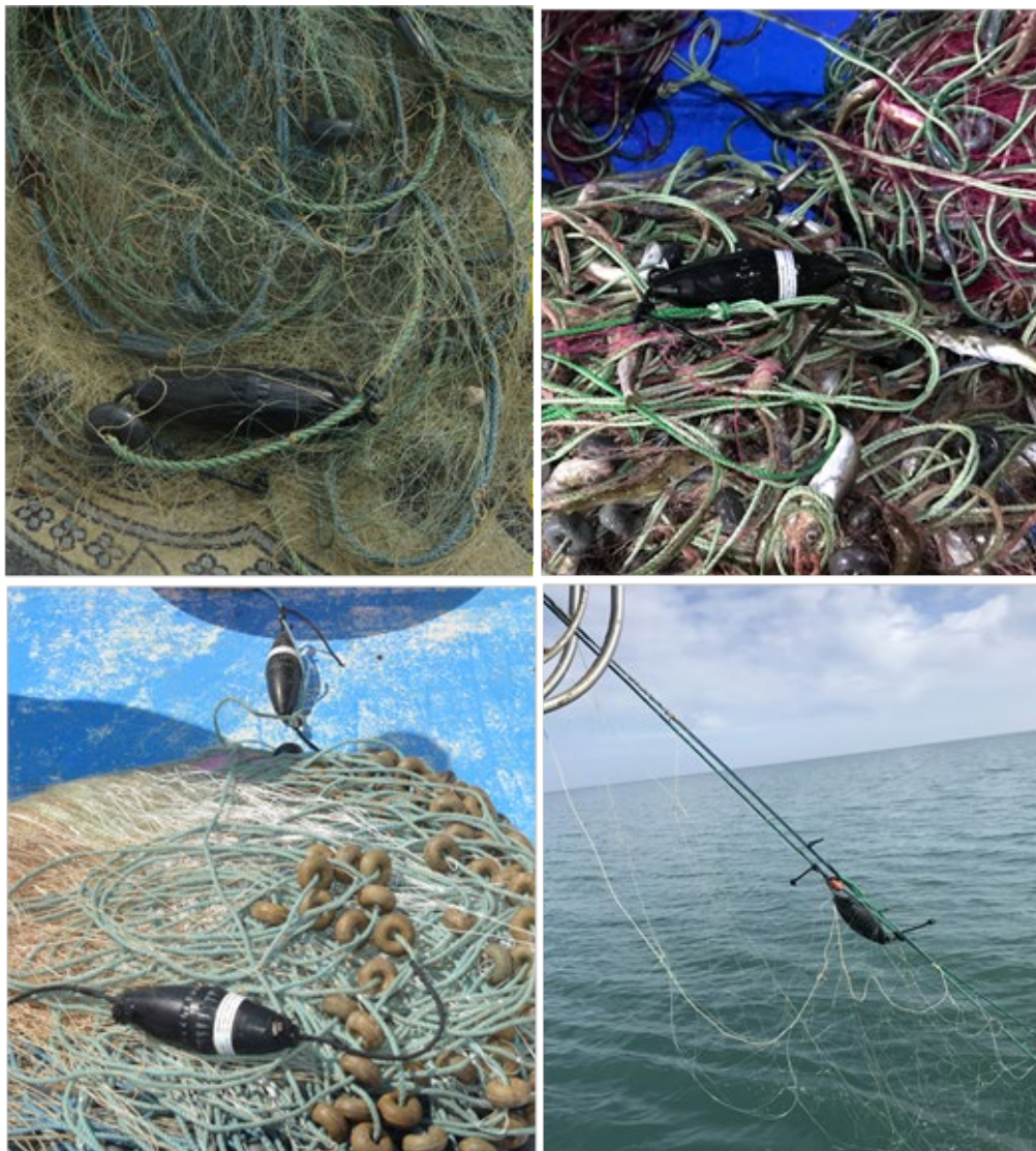
Figure 6. Acoustic device (PAL - Pinger) for prevent of cetacean bycatch in the gillnets
