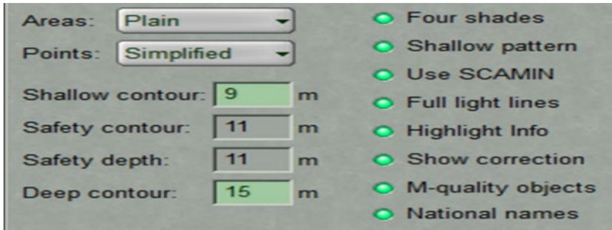
Figure 8. Safety parameters entered into ECDIS
