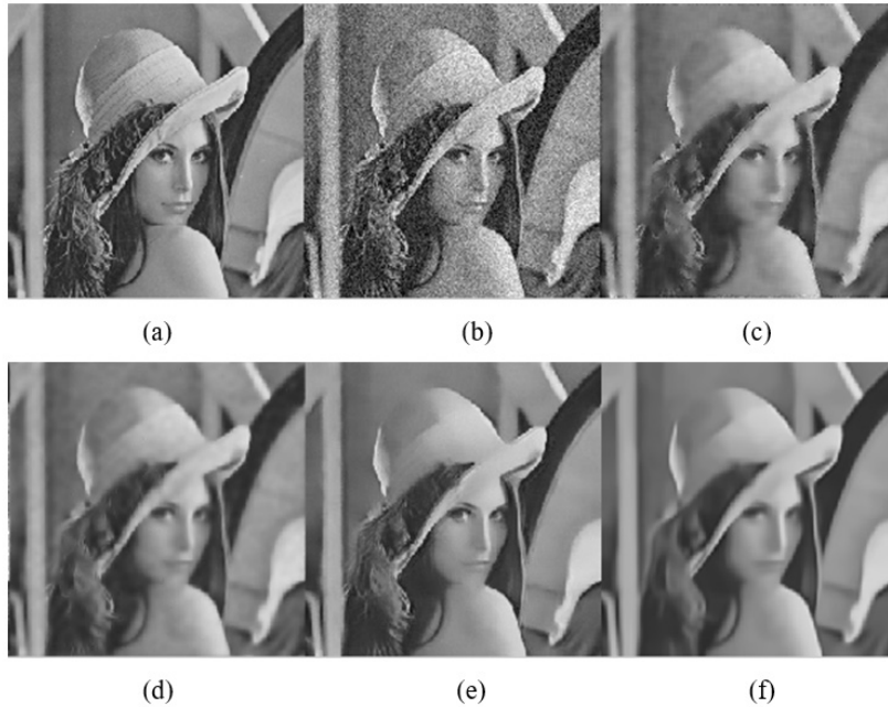
Figure 13. Denoised Lena images ( \sigma = 20 ) (a) Original Lena image (b) Noisy (c) Wiener (d) Wavelet soft thresholding (e) NLM (f) BM3D.
