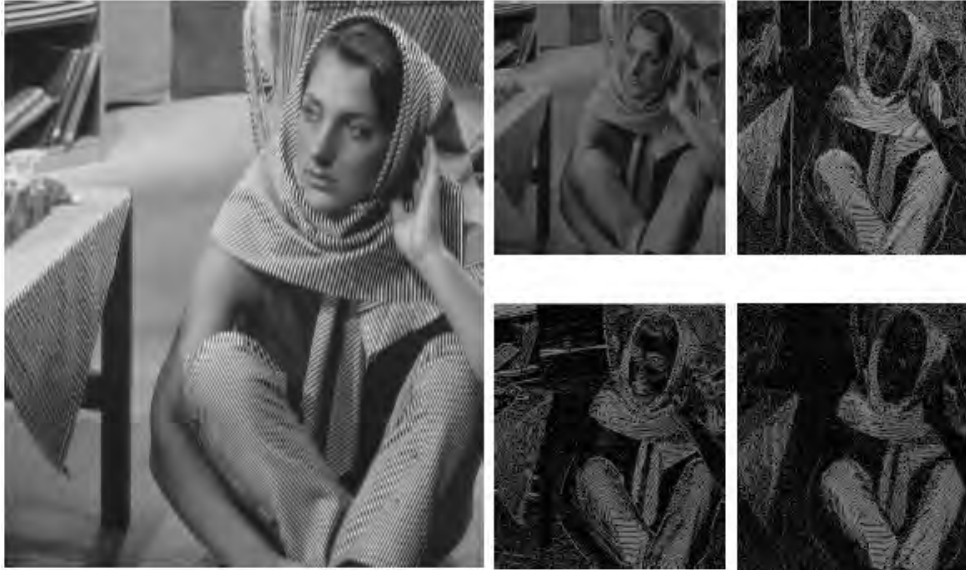
Figure 1. A sample image 'Barbara' and 2-D wavelet decomposition of the image. From top left to bottom right: LL, LH, HL, and HH (detail) subbands.
