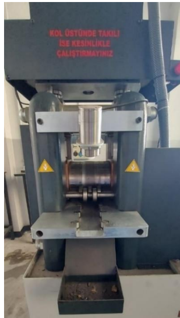
Figure 2. The two-high rolling setup.
