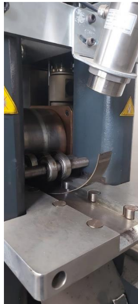
Figure 6. Curvature tendency due to unbalanced residual internal stresses.
