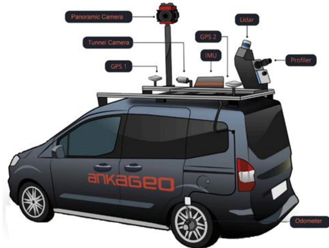
Figure 5. Image of MMS designed by our research team.
