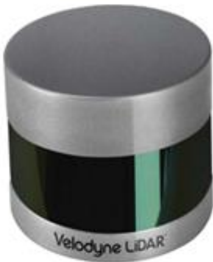
Figure 7. Velodyne VLP-32c in the test measurement.
