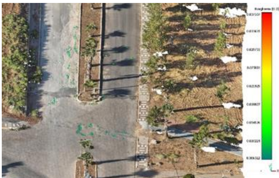
Figure 3. Roughness result of 30 cm kernel size.
