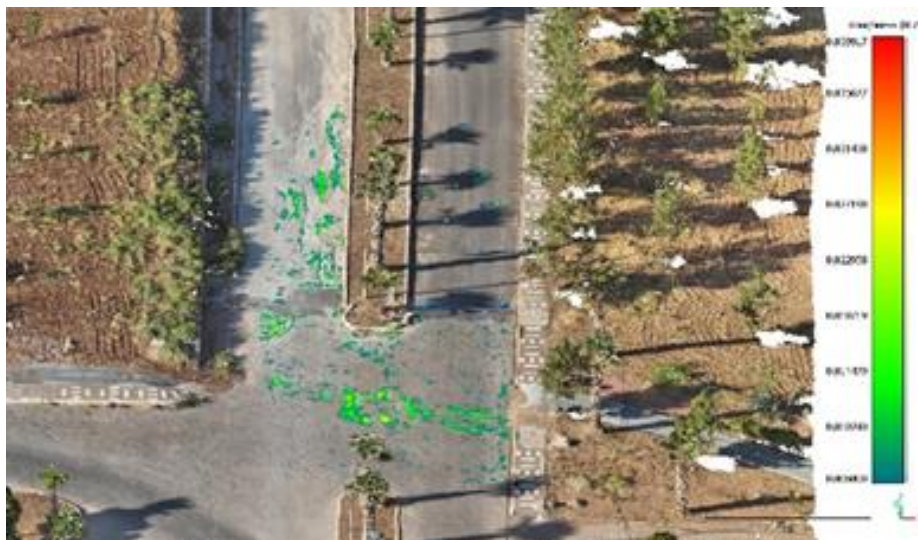
Figure 5. Roughness result of 75 cm kernel.
