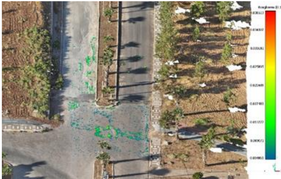
Figure 4. Roughness result of 50 cm kernel.
