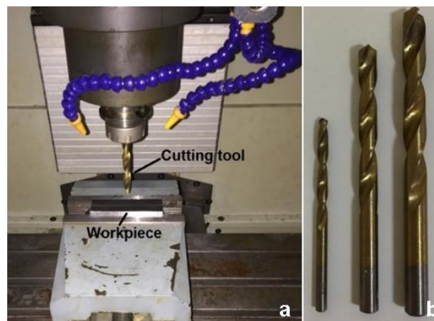
Figure 1. Experimental setup and cutting tools (a. Experimental setup, b. Drills)
