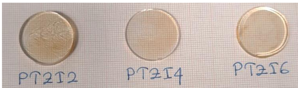
Figure 1. Successfully synthesized In 2 O 3 doped phosphate zinc tellurite glasses
