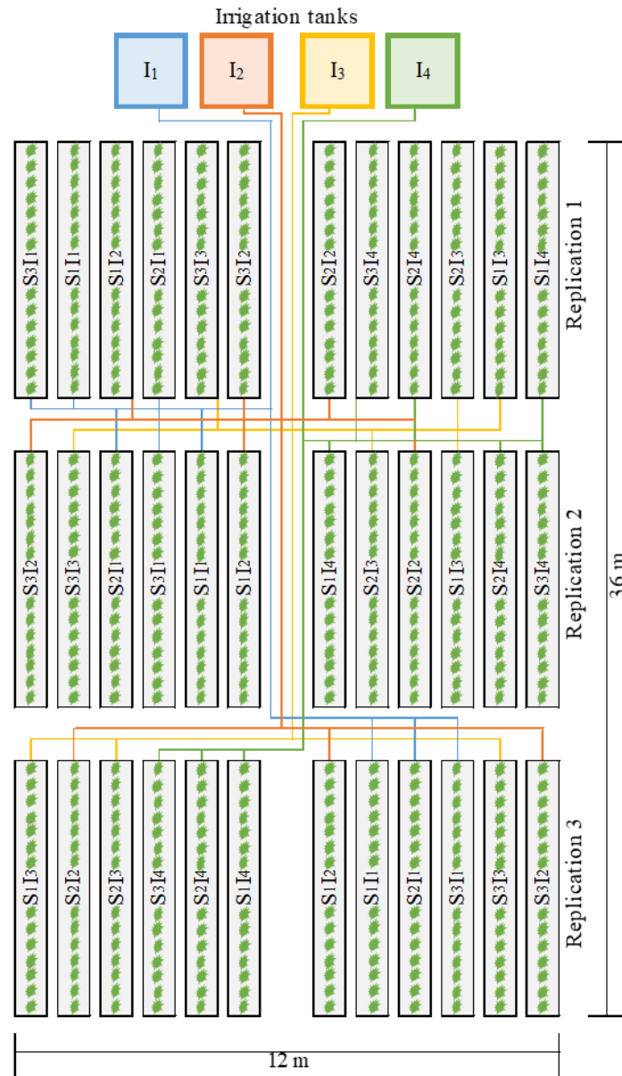
Figure 2- Experimental design used in the study S 1 : 75% cocopeat + 25% perlite, S 2 : 50% peat + 50% perlite, and S 3 : 25% zeolite + 75% peat), I 1 : Irrigated at 100%, I 2 : Irrigated at 75%, I 3 : Irrigated at 50%, and I 4 : Irrigated at 25%
