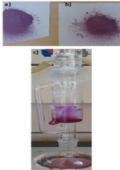
Figure 2. a) Ivy rose extract, b) Velvet red rose extract, c) Production of dyes with the Soxhlet system
