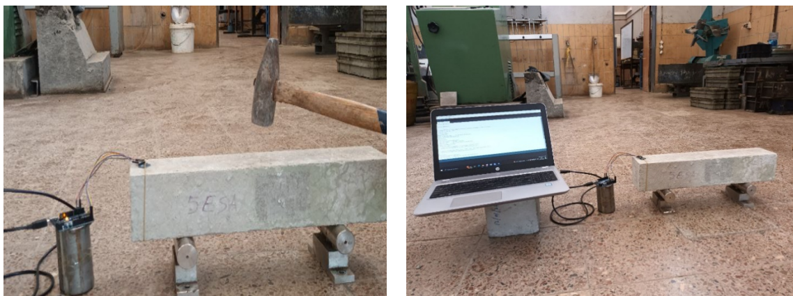
Fig. 4. Experimental Test set-up: accelerometer (Arduino type, MPU-6050) and impactor
