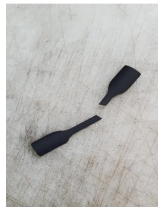
Figure 9. A broken dumb-bell test piece after elongation at break test.
