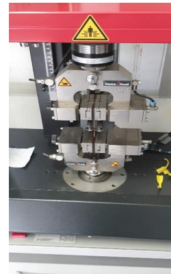
Figure 8. The elongation at break test with a Zwick/Roell Z010 10kN ProLine 739384.
