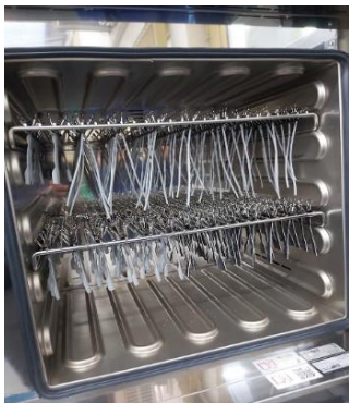
Figure 6. Placing and Suspension of the EPR test pieces inside the ageing oven.
