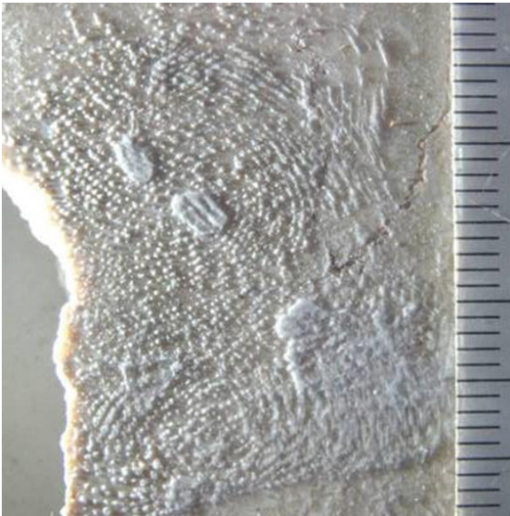
Fig 3. The image of the fingerprint on a marble surface subsequent to cyanoacrylate fuming method application after holding for 3 days
