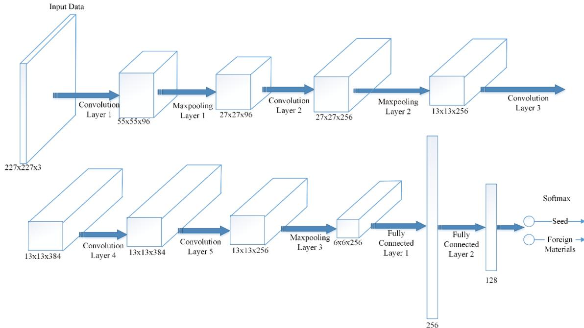
Figure 5. AlexNet architecture.
