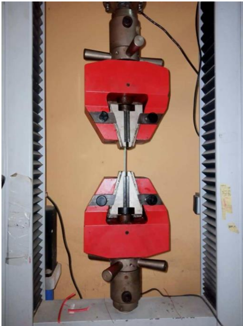
Figure 1. A composite sample undergoing tensile strength test.
