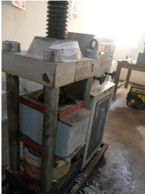
Figure 3. Sandcrete block undergoing compressive strength testing.
