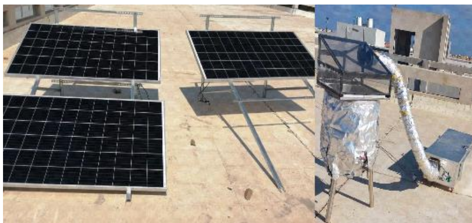
Figure 2. Displays a photograph of the wax melter operated by solar energy.
