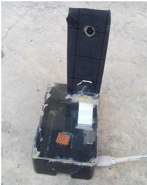
Fig. 7. Prototype of intelligent surveillance system using Faster RCNN
