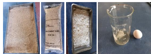
Figure 1. Materials used for the Khorasan mortar a) brick ballast b) standard sand c) lime d) egg white.
