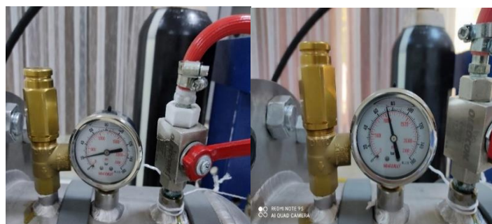
Figure 3. CO 2 reaching supercritical state in the reactor.
