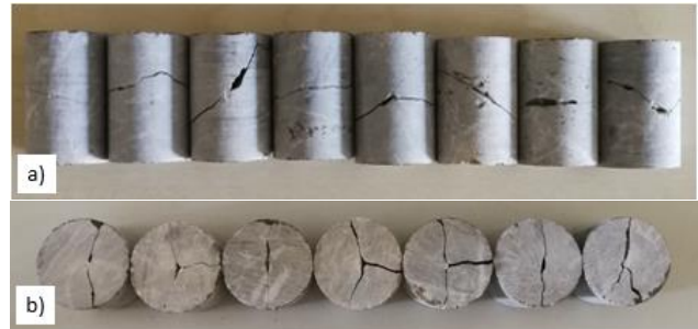
Figure 7. Broken specimens after the PLI tests a) diametral test, b) axial test.
