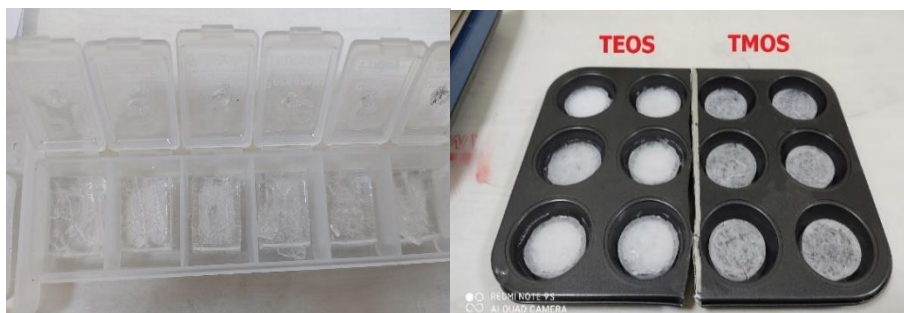
Figure 4. TEOS-TMOS aerogels after drying.
