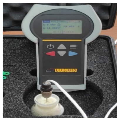
Figure 5. Thermal conductivity tests applied to aerogels.
