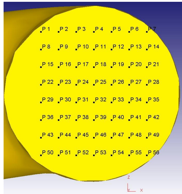
Figure 2. Pattern of points used to determine the effective strain values.
