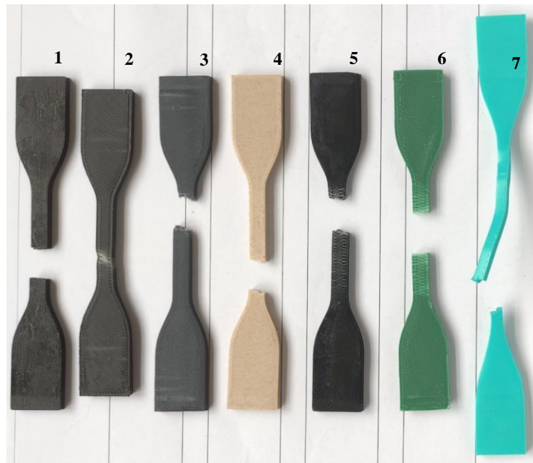
Figure 7. Image of the sample with a 0.1 mm layer thickness after tensile testing
