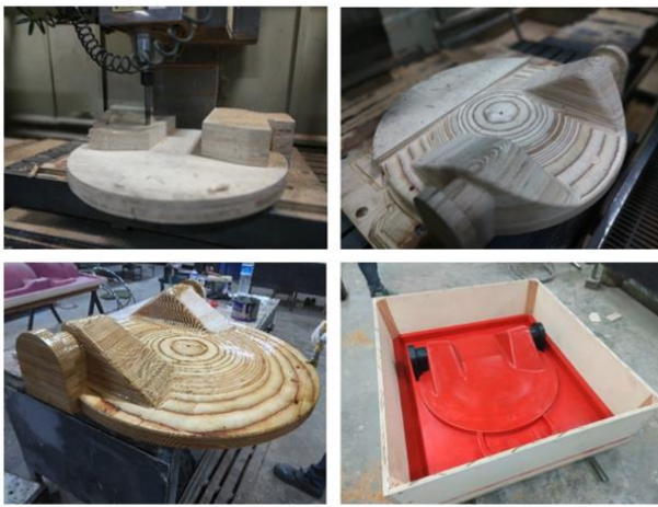
Figure 5. Pre-cast preparations of components' material
