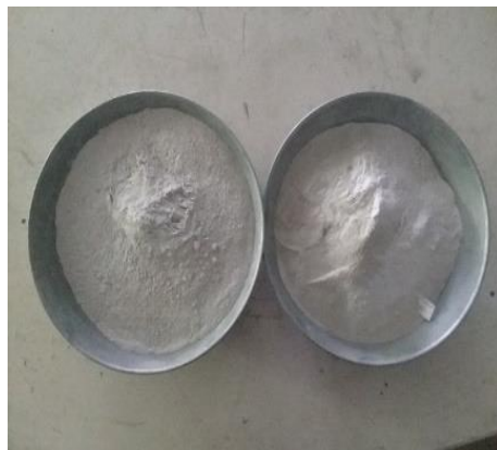
Figure 2. Passing and retaining waste glass through a No. 325 sieve
