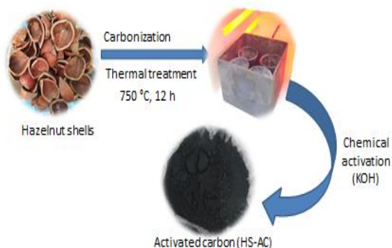
Fig. 1 HS-AC production process
