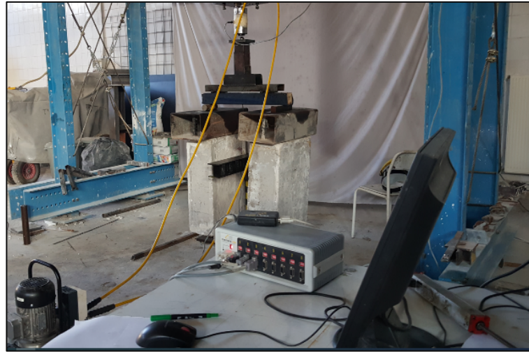
Figure 2. Bending test experimental setup
