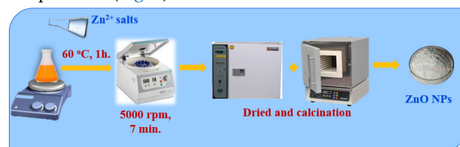
Figure 3. Schematic representation of the preparation steps of ZnO NPs
