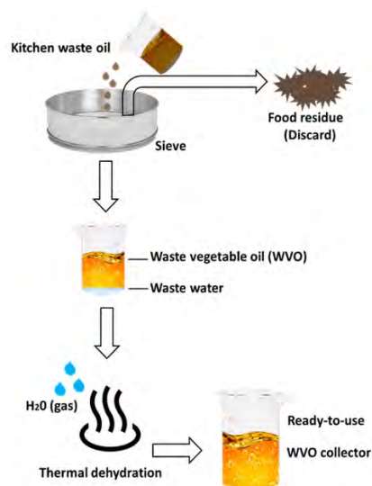
Figure 2. Flowsheet of collector prepared from kitchen waste oil.
