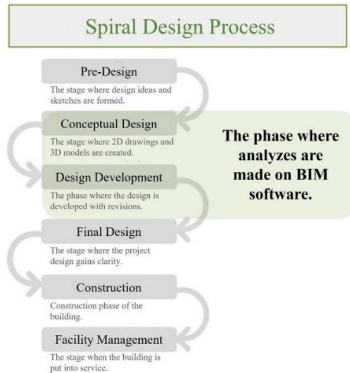
Figure 10. The use of BIM in the processes of high-performance sustainable building design, adapted from Ofluoğlu, 2018 (URL7) (Koçhan & Akin, 2022).
