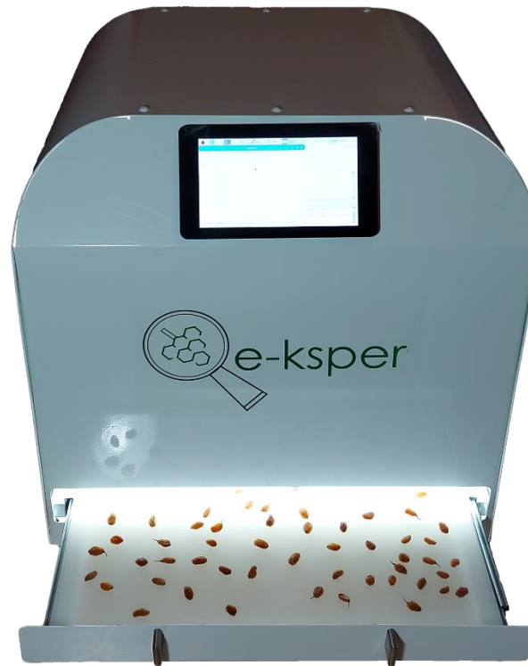
Figure 3. The hardware in which the photos of raisin samples to be evaluated are taken and processed.
