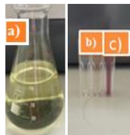
Figure 1. (a) Before microwave treatment, color change of \text{HAuCl}_4 \cdot 3\text{H}_2\text{O} solution and Mulberry leaf extract mixture, (b) and (c) after microwave treatment, purple pink color indicating the formation of Au-NPs.
