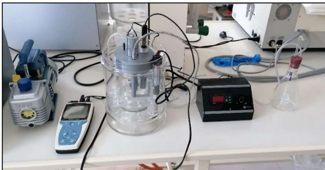
Figure 1: Biogas digester system.
